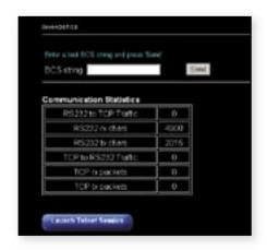
A diagnostics page allows for local and remote diagnostics, and provides a place to launch a Telnet session for sending AutoPatch BCS serial control protocol
